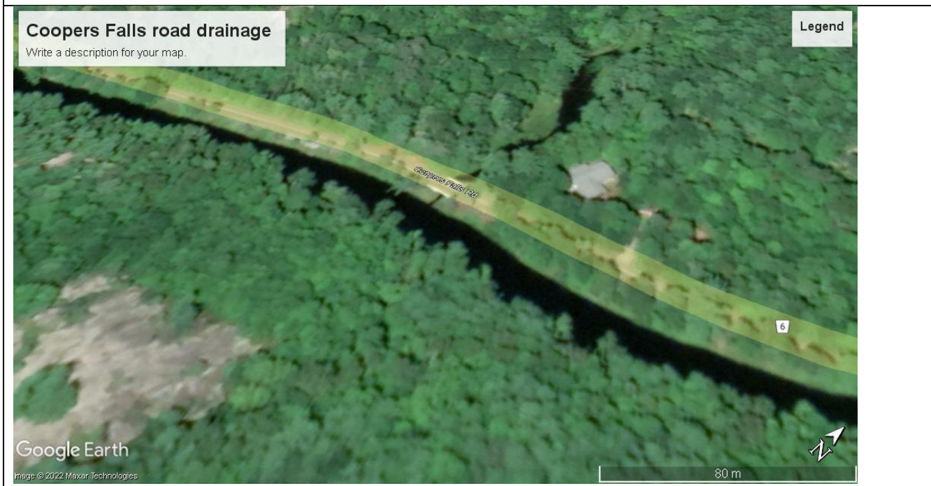
Stream crossing at Coopers Falls road showing location of a box culvert that has potential for wildlife passage located in the connection between the Sadowa Candidate ANSI and QEII provincial park (utm zone 17n 641112 4961373)
