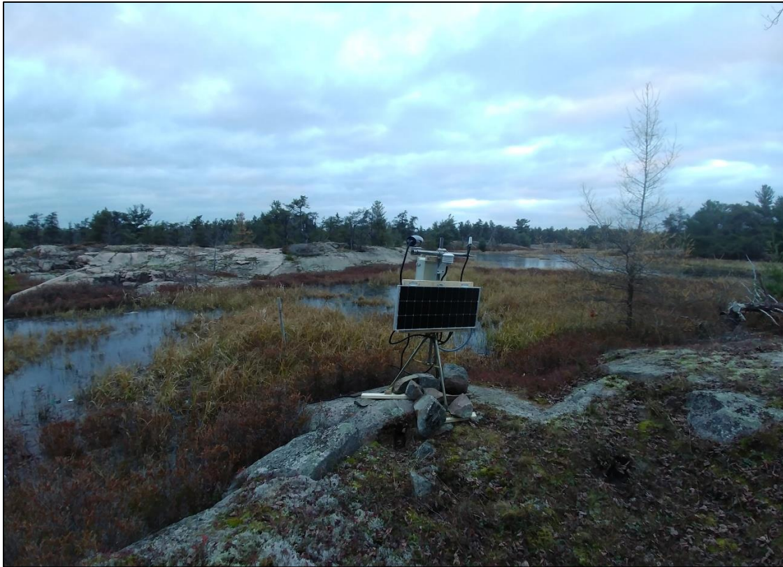
Figure 6. Newly installed micrometeorology station monitoring a confirmed overwintering wetland in the control treatment area.
