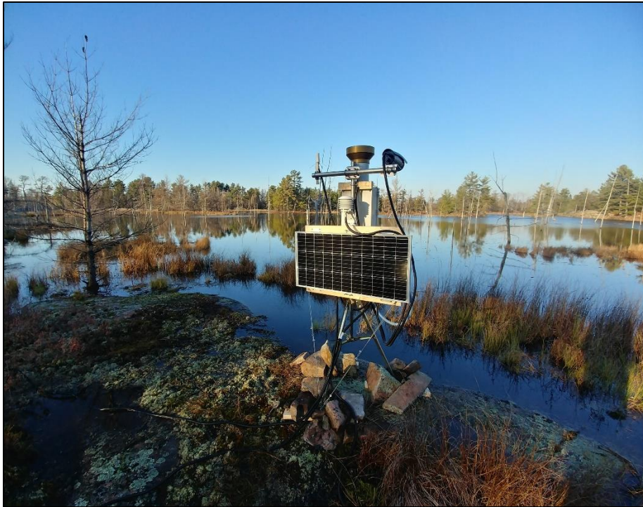
Figure 7. Newly installed micrometeorology station monitoring a confirmed overwintering wetland in the Burn treatment area.
